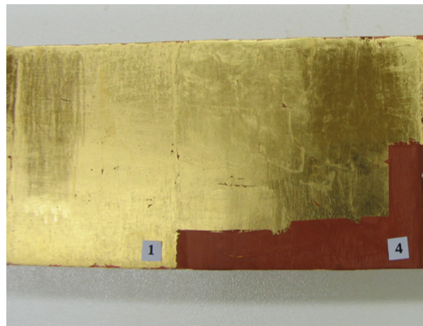
11. Detalj proba 1 i 4 (slijeva nadesno) nakon nanesenih zlatnih listića na bolus, vidljivo je mjestimično poliranje zlatnih listića (fototeka HRZ-a, snimila N. Krstulović, 2015.) Detail of trials 1 and 4 (from left to right) after applying gold leafs over the bole; visible in places is the polishment of gold leafs (Croatian Conservation Institute Photo Archive, photo by N. Krstulović, 2015)
